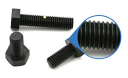
Standard:DIN603, ASME B18.5 Size:M5-M20; 1/4"-1" Length:10mm-500mm Grade:4.8 8.8 10.9 Mark:4.8 8.8 10.9 Material:carbon steel or alloy steel Finish:plain,black,zinc plated ,hdg ,dacroment,geomet and so on.
